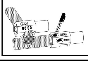
**<u>STEP 3:</u>** Select and assemble required LOKRING tool. Inspect and cycle tool to assure proper function.
